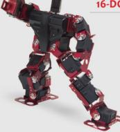
The 16-DOF Robotinno™ Kit is a humanoid robot kit, composed of 16 metal-geared RC servos, aluminum brackets and a Servo Commander™ 16 control board. By using the innoBASIC™ language and Motion Editor utility, users can easily design and implement their own humanoid gait research. This kit is suitable for more advanced hobbyists and for college robotics labs. With its dexterous maneuvering capabilities, it is also very suitable for participation in robotic competitions.
