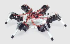
The Hexapodinno™ is 6-legged mechanical beast kit, composed of 18 metal-geared RC servos, PC chassis, aluminum brackets and electronic module boards. By using the innoBASIC™ language and the Motion Editor utility, users have all the tools at their fingertips to implement their own unique beast gait designs. The advanced features of This kit is suitable for more advanced hobbyists and for college robotics labs.
