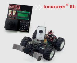
The 4-Wheel-Drived Off-roader is a wheel-type robot kit, composed of 4 DC-motors with off-road tires, DC-motor control board, aluminum chassis, and a BASIC Commander® control board. By using the BASIC Commander® system, users can easily integrate innovati's modules, such as Servo control board for robotic arm application, or Sonar module for obstacle avoidance application, which makes it an excellent platform for intelligent wheel-type robotics research.
