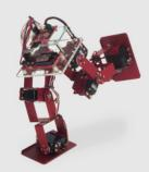
The 6-DOF Bipedinno<sup>™</sup> is a low-cost version of the waist-high two-legged humanoid robot kit, composed of 6 plastic-geared RC servos, PC mounting board, aluminum brackets and a electronic module boards. By using the innoBASIC<sup>™</sup> language and Motion Editor utility, users can easily design and implement their own humanoid gait research. This kit is suitable for more advanced hobbyists and for college robotics labs.
