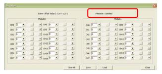
9: Observe the servo requiring adjustment. Press the corresponding arrow button and the servo will rotate in the selected direction. Please make sure the rotational direction is correct. If it rotates in the opposite direction, click the other arrow button to adjust each servo to the middle position in sequence.
