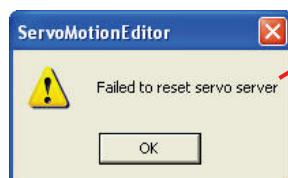
If this message appears, it means that the USB cable is not connected correctly.
