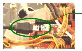
The connectors at the two ends of the USB line are of different sizes, so please connect the smaller one to the BASIC Commander<sup>®</sup>.
