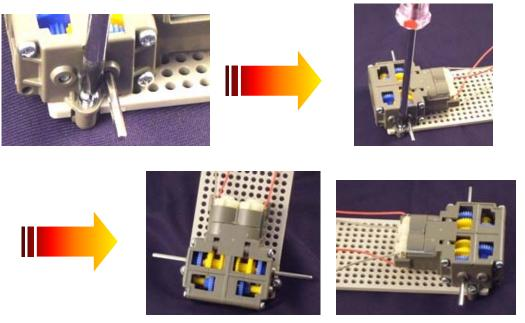
v. Install the wheels at the bottom chassis: The pins and the wheels should be assembled in the ways as shown in the following figures. Fix the three wheels on the backside of the PC board.
