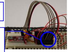
v. Plug the Jumper as the power switch to complete the assembly of the Tankbot.
