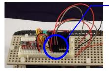
4 motor power wires: 20a, 21a, 22a and 23a
