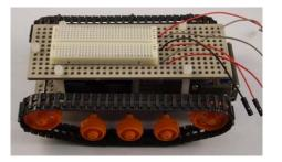
ii. Plug the BC1, Motor Runner B, jumper wires, and pin headers on the breadboard according to their arrangements shown in the following figure. BC1 should be located at the pin coordinate 1c-12c and 1g-12g. Motor Runner A should be located at the pin coordinate 18e-29e.
