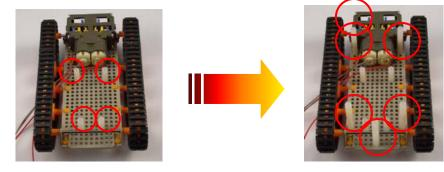
x. Install the battery box: In order to avoid short circuits, it is recommended not to install the battery cells in the beginning.
