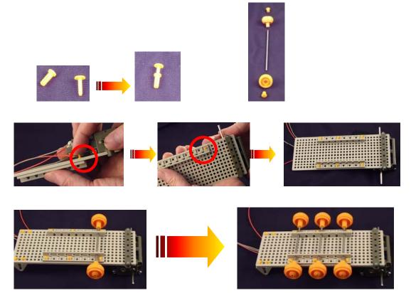
vi. Install the front and rear wheels: Install the rear wheels (smooth wheels) on the triangular rack on the front side. Install the front wheels (saw-tooth wheels) into the metal axle on the gearbox.
