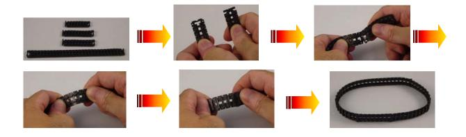
viii. Install the caterpillar band: Install the caterpillar bands at the two sides as shown in the figure.
