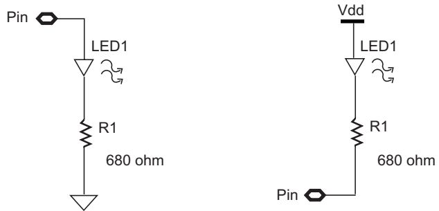
Figure 6-4 Illuminating a small LED using HIGH and LOW commands
