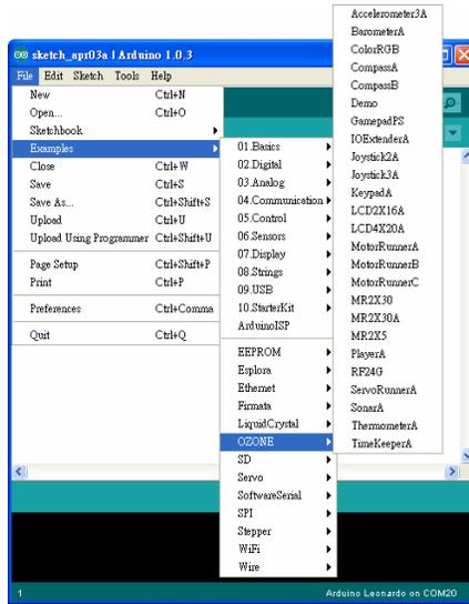
After the program is loaded, you can see the code in the editing window. Compile and upload to the Ozone board. Some example programs can be found in the Appendix section.
