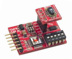
**Product Overview:** With the connection through cmdBUS to BASIC Commander, the user can use simple commands to obtain the present temperature and humidity from Innovati's Thermometer A module and then calculate the dew point value. Through simple commands, the module can perform functions such as automatic measurements, alarms on changes, etc.
