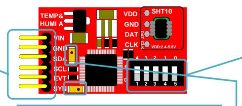
From the top to the bottom: Command Indicator: The blinking light indicates the module and the SBC are transmitting/receiving data. Event Indicator: The blinking light indicates that the module generates an event.
