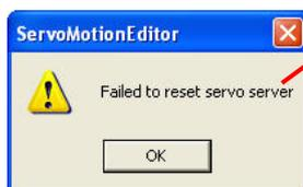
If this message appears, it means that the USB line is not connected correctly.
