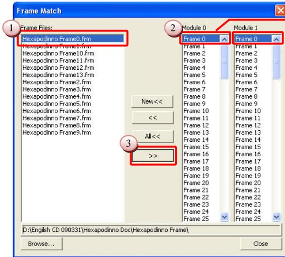
Before clicking the “>>” button to download the motion file into the module, please make sure that the “Frame 0” under the Module 0 and Module 1 has been selected and highlighted.
