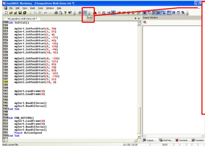
If the user is not sure about the function of each button, the user can move the mouse pointer over the image. After a while, the English name will automatically appear. After click the "Build" button, the program will be downloaded into the BASIC Commander and stored automatically. According to the layout, the "Build" button may appear at different position.
