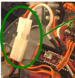
While connecting the power cord, please notice the polarity. Connect the two red wires together.
