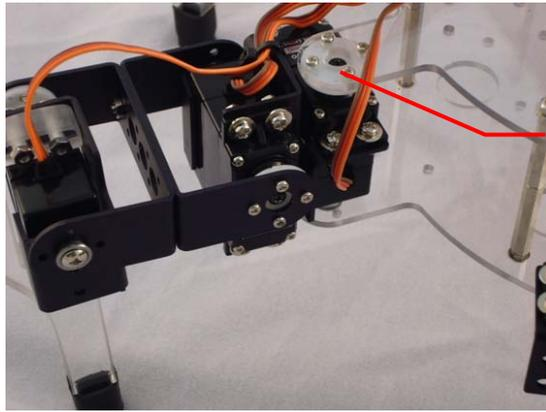
While fixing servomotors, let the joint form a reverse L against the ground, with the supporting leg positioned on the extension of the line that joins the center point and the inner joint.
