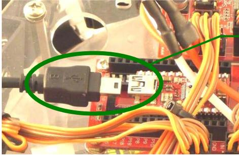
The connectors at the two ends of the USB line are of different sizes, so please connect the smaller one to the BASIC Commander®.
