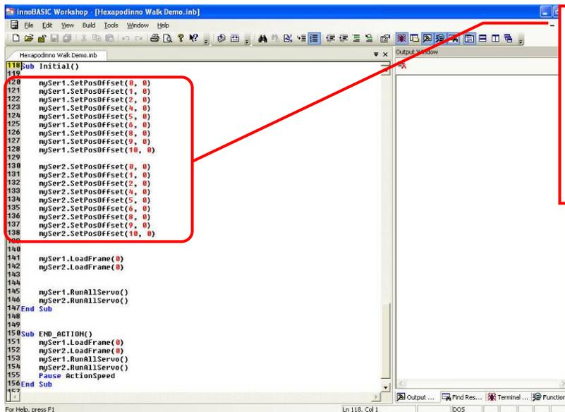
The number on the left side represents the line number of the program. The Function starts at "Sub" and ends at "End Sub" within which the operations are defined to store the fine tune values into the module. At the beginning of each program, it is necessary to set the fine tune values.
