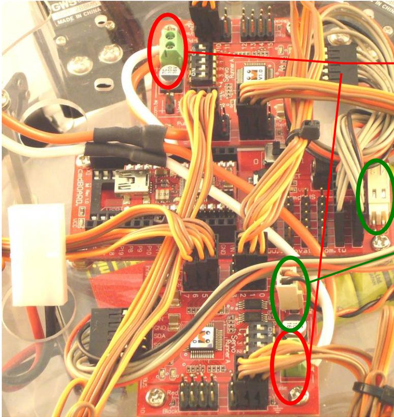
Please connect the two ends of the power line to the green power headers on two Servo Runner A's. Please use a screwdriver to loosen the two small screws. After inserting the wires, tighten the two screws to fix the wires.
