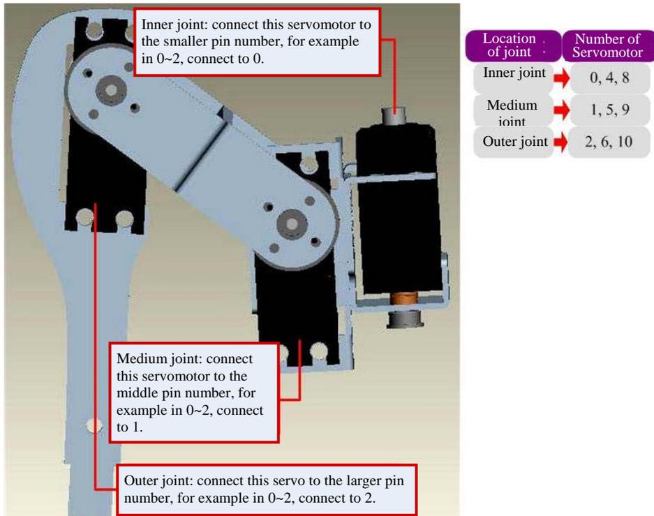
*※ Each Servo Runner A has its own servomotor ID. Please notice that the orange (white) wire is the signal wire; the red wire is the power cord, and the brown (black) is the ground wire. Please connect them according to the positions marked on the module to avoid damage to the module.*
