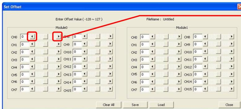
The left/right arrow buttons can be used to rotate the servomotor clockwise or counterclockwise. Please observe the rotation of the servomotor to the required central position. Then adjust the next servomotor.
