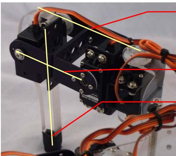
Adjust the Servo inner joint so that extension of the line linking the supporting leg and center of motor disk, as shown in the photo, passes through center of Top Board.
