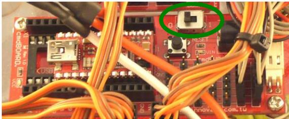
**B\_3. Connect the power line of the servomotor to the power supply (Please make sure that the voltage and current from the power supply are within the range required by the servomotor. After connecting the power line, the servomotor will make a transient motion due to receiving the switch surge, which is normal. While connecting the power cord, please pay attention not to place your hands within the space where the servomotor will move into to avoid being clamped.)**
