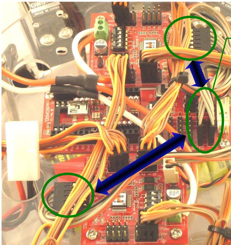
The two cmdBUS™ are connected to Servo Runner A from Command Board. Please note that no matter Command Board or Servo Runner A is connected, the user should pay attention to the polarity.
