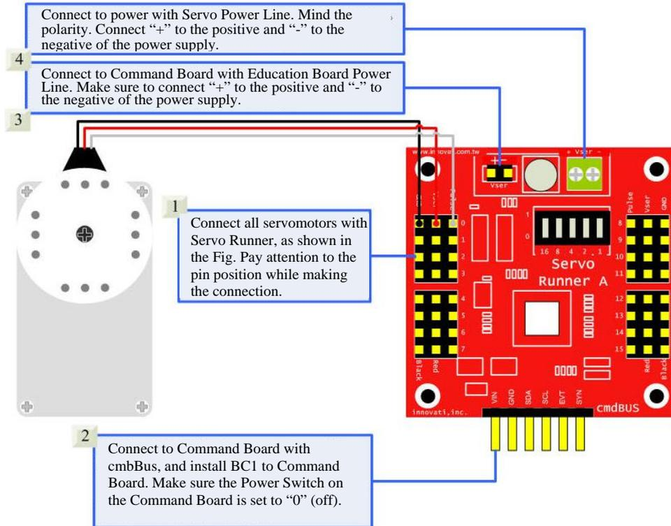
※When the Command Board or Education Board shares the power supply with Servo Runner A, please notice that the voltage of this kit should be 6V (please refer to Notices). It is recommended to use a voltage regulator to ensure that the voltage is within the safe range.
