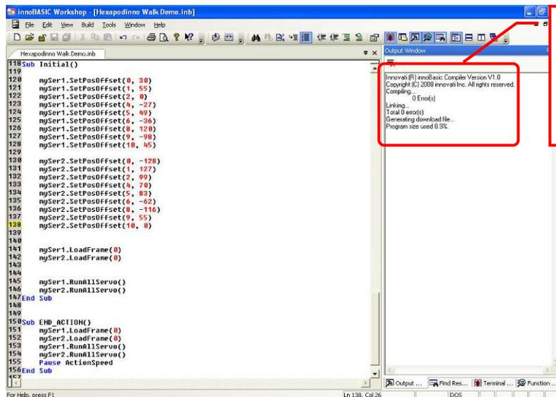
After the download is complete, the output window will display the used memory space. If there is any error, it will be displayed in the output window. Please make sure that no error is displayed in the output window.
