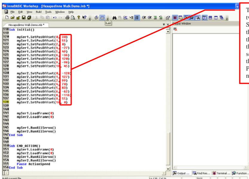
The SetPosOffset command has two parameters: one is the Servomotor ID and the other is the fine tune value. Please enter the fine tune value according to the value recorded for each servomotor ID. The number in the figure is arbitrarily defined, Please do not enter the same number as shown in the figure.
