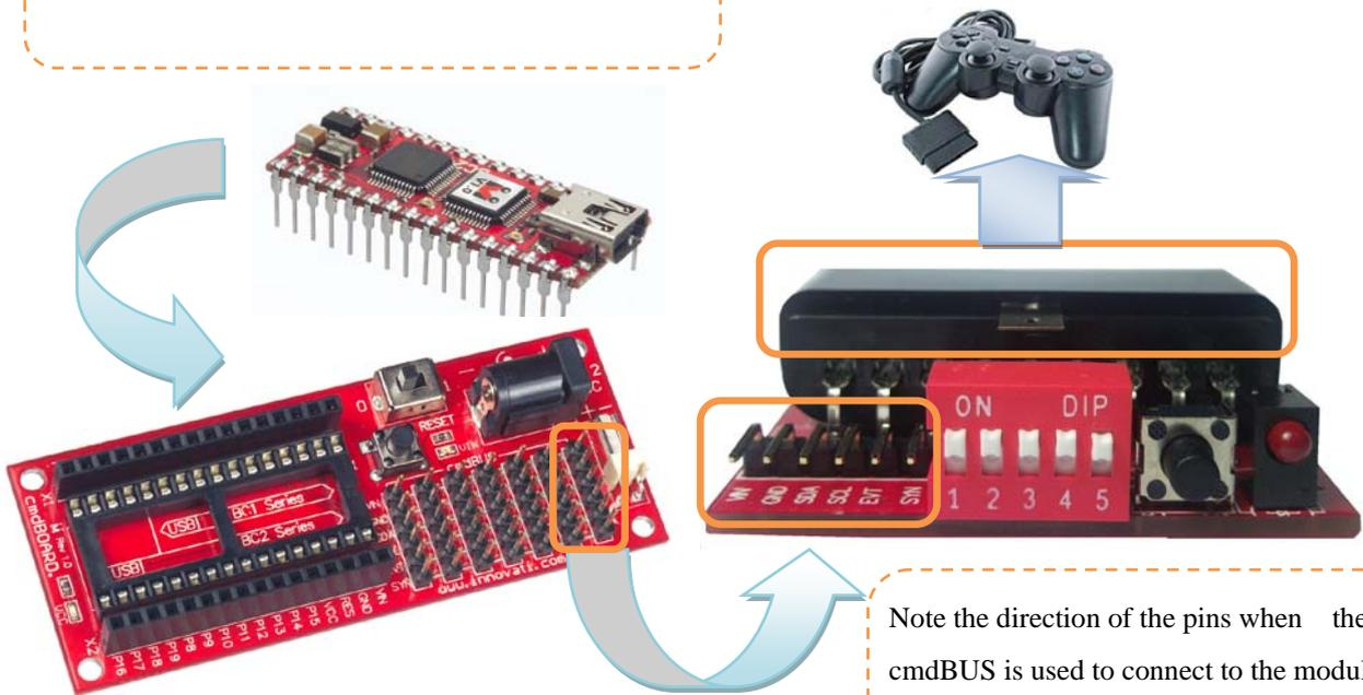
Note the direction of the pins when the cmdBUS is used to connect to the module.
